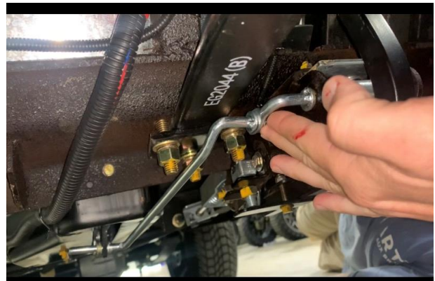
#4 verify if arm is locked against the leaf spring causing throttle pedal to remain fully engaged.
